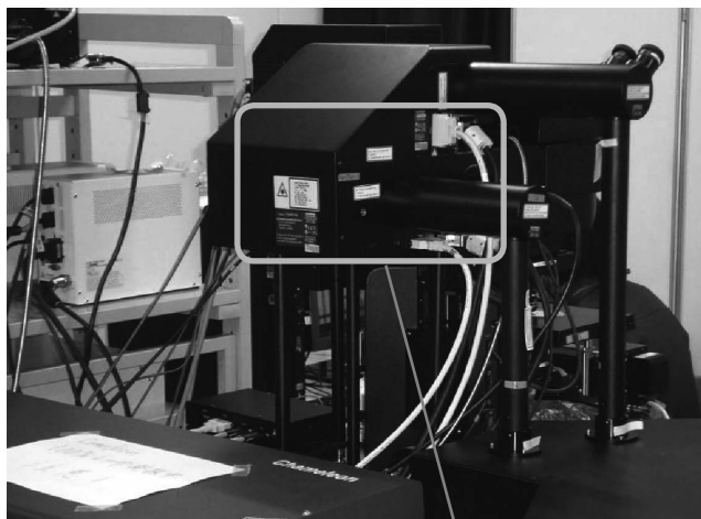
Hybrid scanning unit for MPE (FV30-HSUMP)
