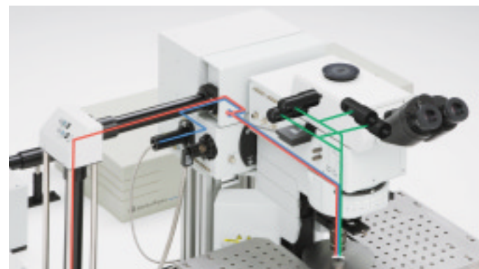
Red: IR pulsed laser (for stimulation/observation), Blue: Visible light laser, Green: Fluorescent light
